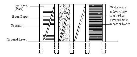
Fig.2 Poteaux en Terre Construction (Source:http://www.cr.nps.gov/seac/gabes/index.htm)
